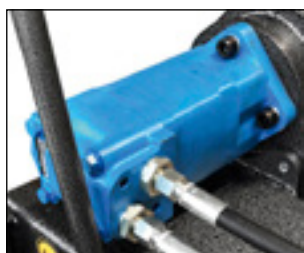
Rotation of the centering claw by hydraulic drive
