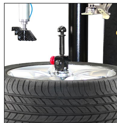
Unblocking by expansion with the rocker lever
