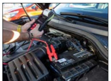
The battery tester with integrated printer is compatible with 6V / 12V / 24V battery tests.
