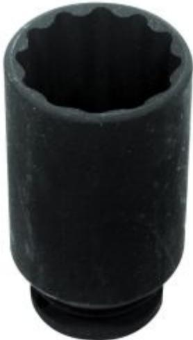
**Libellé article** DOUILLE CHOC ECROU MOYEU VAG 12 PANS Ø36mm 1/2" L.85mm
